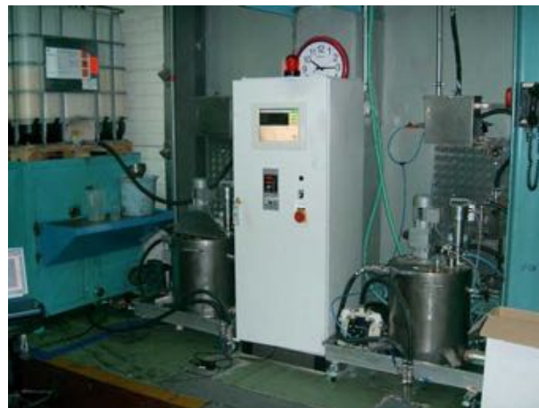
LC1 control cabinet with PC and software, different tank sets for coating
