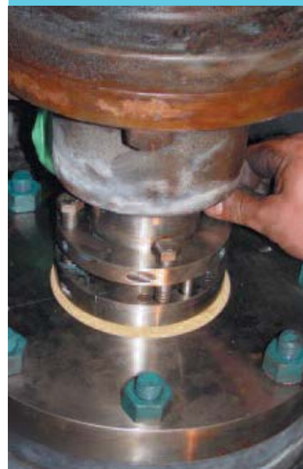
Split OFS seal on 30 top-entry agitator
